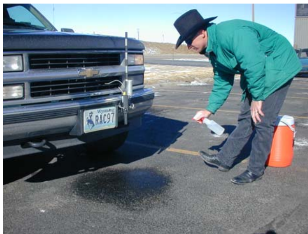
Figure 5. Method to determine effect of differential emissivity on accuracy of temperature measurements.
